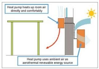
**Figure 2.** Heat pump with indoor heating unit below window for comfort (warm air on the floor) and efficiency (drawing convection flow cooled at glass surface) [5]
